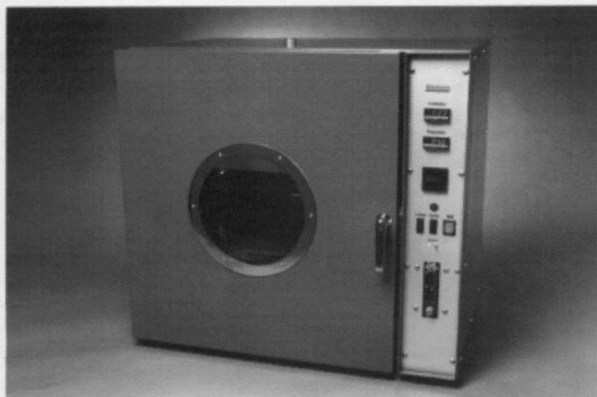
Fig. 13. Cabinet ageing oven EB 04.
