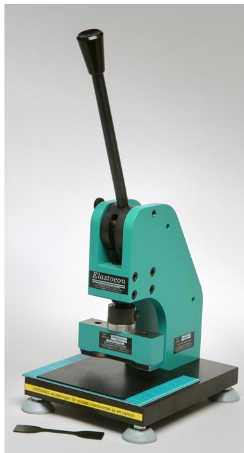
Manual cutting press, EP 08.
