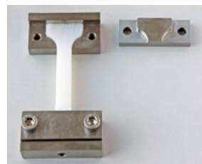
EB 18-II.01 Clamp for creep tests in tension with 50 mm gauge length.
