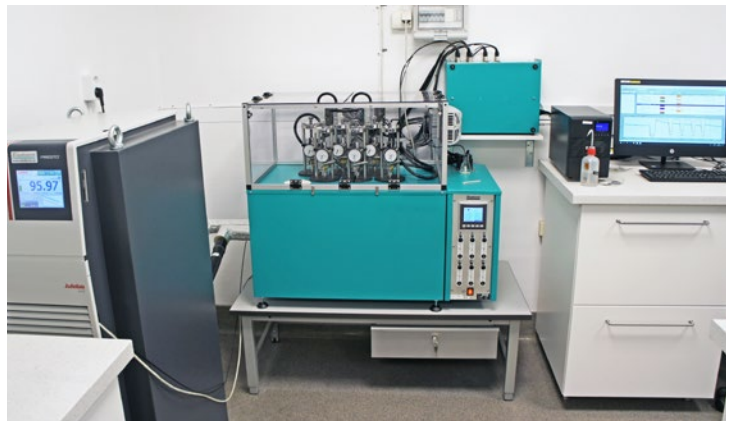
Relaxation system EB 17 with temperature cycling.
