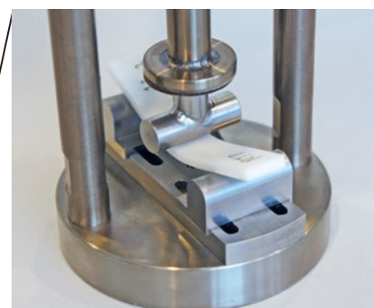
EB 02.29 Fixture for bending test with 3-point loading.
