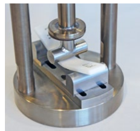
EB 02.29 Fixture for flexural creep by 3-point loading, according to ISO 899-2.
