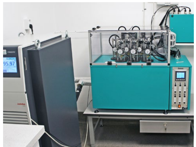
Temperature cycling oven EB 17 for relaxation tests with 6 cells with the same temperature and cycling between subzero to elevated temperature. The oven is placed on the EB 17.04 table, with the liquid circulator to the left.
