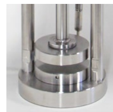
EB 02.29 Fixture for bending test with 3-point loading.
