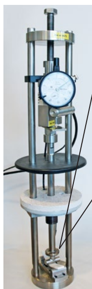
EB 02.29 Fixture for bending test with 3-point loading.
