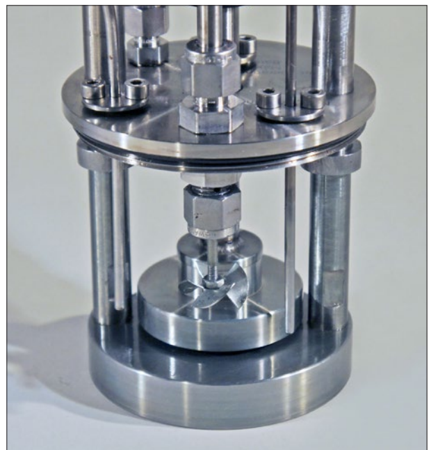
The ALE-test rig has a propeller for mixing in the air in the liquid, as well as for stirring the liquid in the container.
