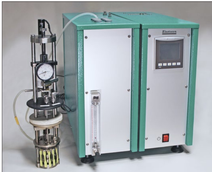
The ALE-test system relaxation rig and the control box with a PLC touch screen.
