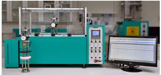
Stress relaxation test system for continuous measurement of rubber in either compression or tension according to ISO 3384 and ISO 6914.
