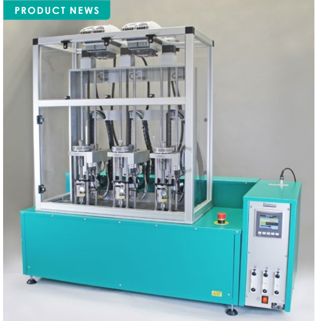
Automatic relaxation and creep tester with temperature cycling, EB 32.
