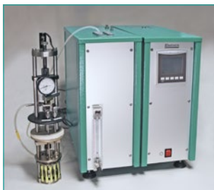
The ALE-test system relaxation rig and the control box with a PLC touch screen
