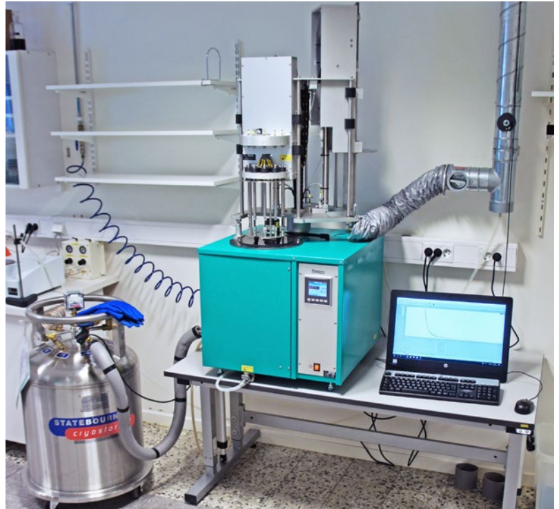
A TR and Gehman Tester combined using the same base unit with a rig changing system, on the adjustable table ET 01.08. To the left the automatic cooling with liquid nitrogen, ET 01.02, which consists of a cryogenic vessel for the storing of liquid nitrogen and a special valve and hose that is needed for the connection between the vessel and the low temperature tester.
