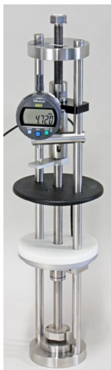
The test rig EV 09 is adapted for Low Temperature compression set.
