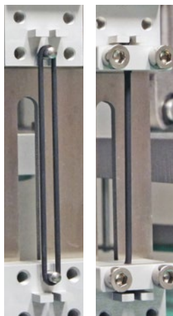
Grips for O-rings (both whole and cut) is an option for the TR Tester.
