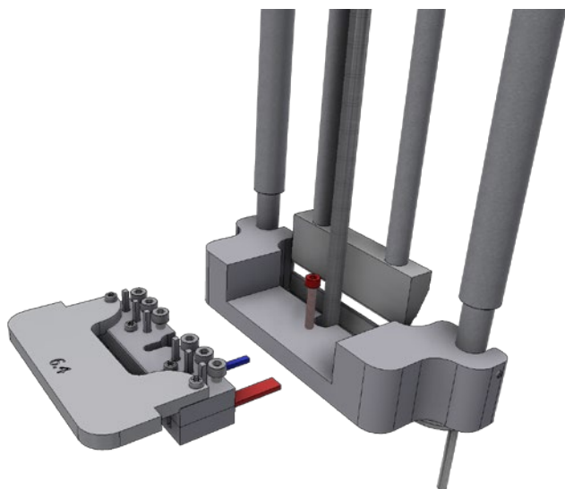
Specimen holder with a distance bracket for different material thickness according to ASTM D2137 and ISO 4646. In this example, the distance bracket is 6,4 mm.
