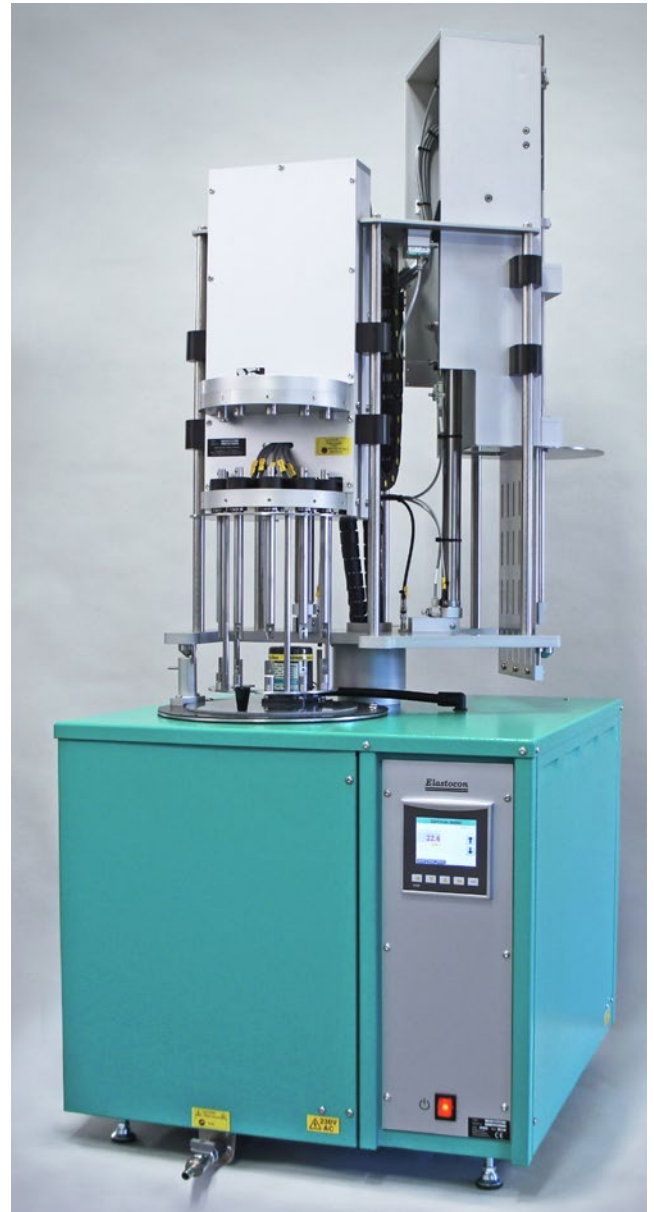
Automatic cooling with liquid nitrogen, ET 01.02.
