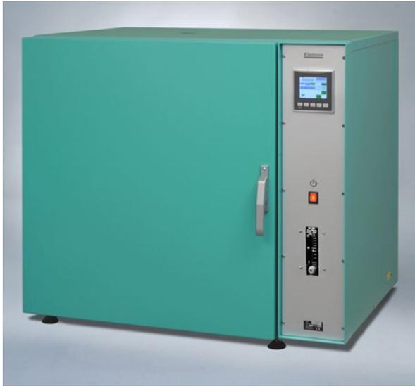
The **EB 04-II cabinet oven** has low air speed and a flow meter that can be set between 3 to 20 changes per hour, which meets the requirements in ISO 188 method A. It also performs well inside the apparatus requirements in IEC 60811-401, IEC 60216-4-1 and other equivalent standards.
