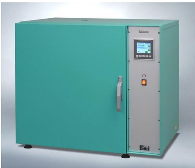
The **EB 12-II cabinet oven** has high air speed with laminar flow from bottom to top, and a factory set throttle to give a fixed air exchange rate of 7 (default) or 14 changes per hour, which meets the requirements in ISO 188 method B.
