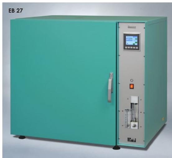
The EB 27 cabinet oven has 2 flow meters to cover the exchange rates between 3 to 200 changes per hour, but still with low air speed inside the chamber. The oven meets the requirements in ISO 188 method A, IEC 60811-401, IEC 60216-4-1, ASTM D5423 type 1 and 2, ASTM E145 type IIA and ASTM D573. The useful volume is 120 litres.
