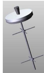
One sample holder per cell is included with the cell ovens.
