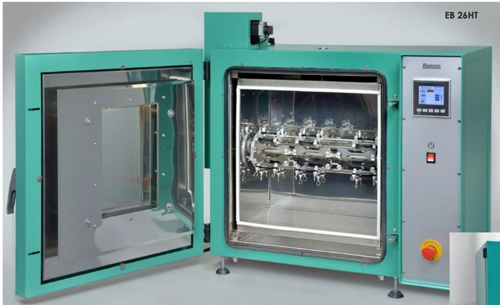
In addition to the carousel the EB 26HT cabinet oven is also equipped with a window in the door, lighting inside the chamber and a door sensor that turns off the fan, heating and carousel when the door opens.
