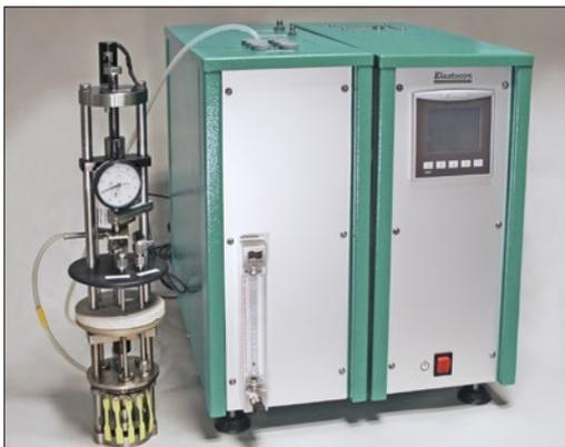
*The ALE-test system relaxation rig and the control box with a PLC touch screen. The ALE-test system is purchased as a complement/accessory for use with a stress relaxation system for continuous testing. The ALE rig has a propeller for mixing in the air in the liquid, as well as for stirring the liquid in the container.*
